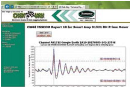
Figure 01: GOOD BUMP - Data captured from the vehicle shows an isolated bump and the suspension is working well.
